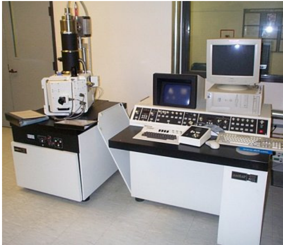
Figure 32. (left) The Amray 1830 Scanning Electron Microscope is used to image devices. (right) SEM image of a device that has been prepared for indium bump deposition.
